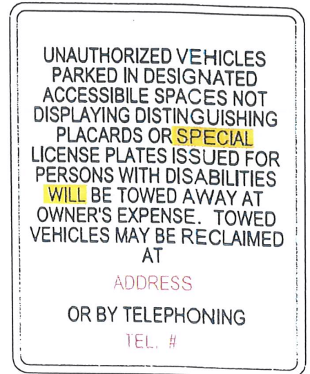
CBC 11B-502.8.2 Tow Away Sign
